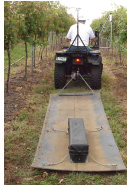
'On-the-go' soil sensing using an EM38.
