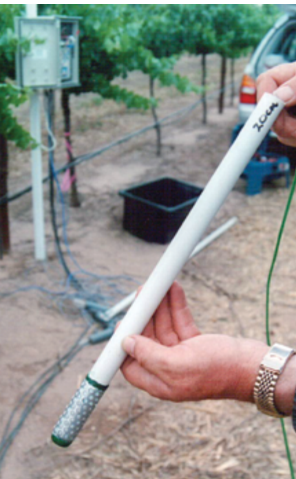
Installing a gypsum block to measure soil water tension.
